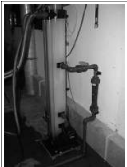
Figure 7. Ozone is added through a venturi pump on the protein skimmer. Protein skimmer has a capacity up to 50 litre/min and have two venturi pumps which deliver 100 mg \text{O}_3 /hour from the two pumps (Sander Ozonisorator 100).
