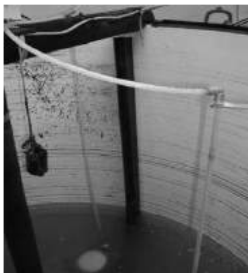
Figure 24. Walls and cleaning arm after 65 days rotifers culture.
